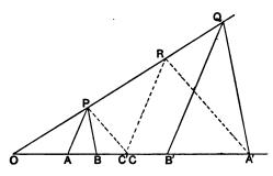
Let A, A'; B, B'; be two pairs of points on a straight line. Through A and B draw any two lines AP, BP intersecting in P; and through A', B' draw A'Q, B'Q parallel to BP, AP respectively, meeting in Q. Let PQ meet AB in O.
